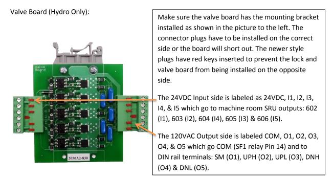
The orientation of both the valve and lock boards on the controller mounting rail is as follows:
