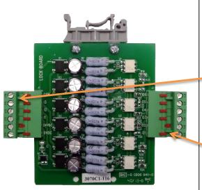
Make sure the Lock board has the mounting bracket installed as shown in the picture to the left. The connector plugs have to be installed on the correct side or the board will short out. The newer style plugs have red keys inserted to prevent the lock and valve board from being installed on the opposite side.
