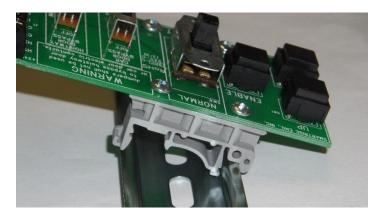
7. Rotate the new board down onto the rail and snap it into place.
