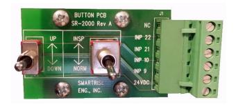
4. Remove the Inspection board from the rail by reaching behind the plug side and prying up on the two grey tabs that attach it to the rail.
