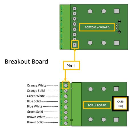
Replacing the breakout board is a simple process that doesn't require removing any wiring.
