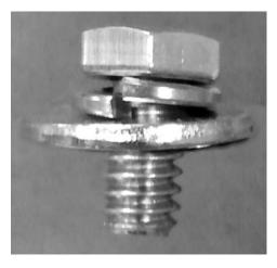
Take out the six (6) bolts, flat washers and lock washers and assemble them as shown.
